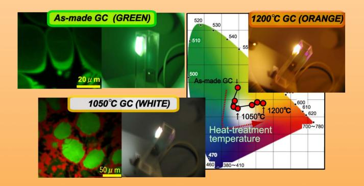
Preparation and luminescent properties of  $Eu^{2+}$ -activated glass ceramic phosphor precipitated with  $\beta$ -Ca<sub>2</sub>SiO<sub>4</sub> and Ca<sub>3</sub>Si<sub>2</sub>O<sub>7</sub> (T. Nakanishi and S. Tanabe, p. 919)
